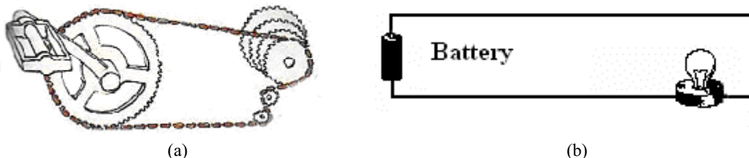
Figure 1. Simile of the circulation of electrical current as the movement of a bicycle chain.
