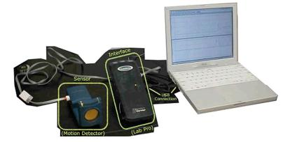
Figure 2: Technology setup consisting of sensor, interface and laptop computer connected via USB connection
