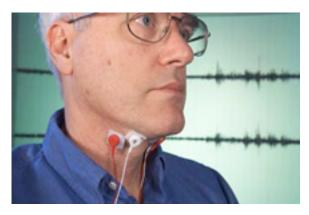
To make this technology work, small electrodes are placed on the throat near the larynx. The signal that is created by thinking is captured and recorded. The list of recorded nerve patterns creates a type of dictionary that a computer remembers. So far, the system is able to recognize a few words, and only words spoken by a particular voice. As the system improves, it will be able to recognize more words and more speech patterns.
