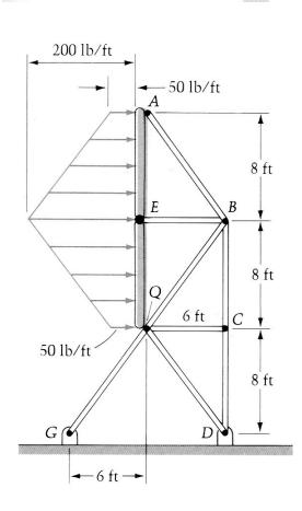
3. The structure to the left represents an edge view of a billboard. The distributed force shown models the wind force. Find the force in member BC.
