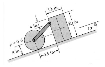
4. In the figure at left, the block weighs 26 lbs and is connected to the roller by a light rod. If the coefficient of static friction between all surfaces of contact is 0.6, what is the maximum allowed weight of the roller for equilibrium?
