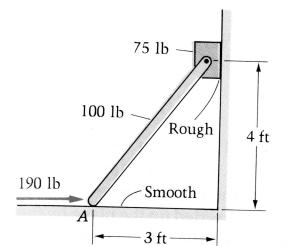
5. What is the minimum coefficient of static friction between the block and the wall for equilibrium?
