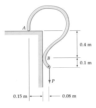
6. The hook shown rests against a rough surface at *A* and a smooth wall at *B*. What is the minimum coefficient of static friction at *A* that will prevent the hook from slipping, regardless of the size of the load *P*? How would you change the 0.4 m dimension to require a smaller friction coefficient of 0.2?
