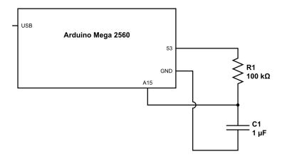
Pin 53 is a digital pin, which we will configure as an output, capable of giving either +5 V (HIGH) or 0 V (LOW). Pin A15 is one of the analog input pins and is capable of measuring analog voltages (0 - 5V).
