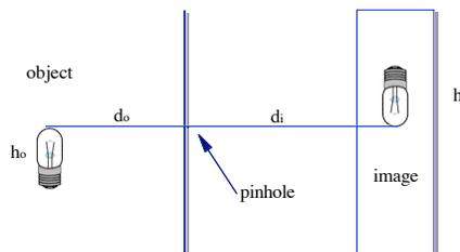
**Step 1. Identify the problem to be solved.** A physicist wants to experimentally determine the relationships associated with image formation in a pinhole camera (see the image above). The physicist seeks to find all the relationships between the height of an object,  $h_o$ , the height of its image,  $h_i$ , the distance of the object,  $d_o$ , and the distance of the image,  $d_i$ , as measured from the pinhole.
